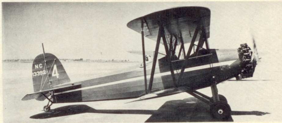
Installation of a nine-cylinder, 220 h.p. Lycoming engine converted 203A models to 203B. This is the second school-built 203. In 1941, the Boeing School abandoned its traditional green-gray-orange color scheme and adopted overall Cadmium red with white trim.
